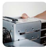
Easy-assembly internal drive cage for 4 x 3.5" HDDs
